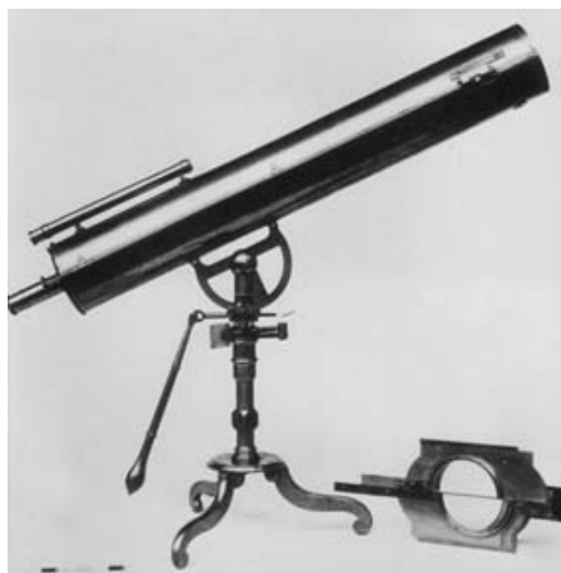
Figure 1. Gregorian reflector 1900-136, by Short, with object-glass micrometer (Courtesy: Science Museum, Science and Society Picture Library).
